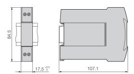
Fig. 6. SINEAX SI 815-5.... (housing **N17**) clipped onto a top-hat rail  $(35 \times 7.5 \text{ or } 35 \times 15 \text{ mm}, \text{ acc. to EN } 50 \text{ } 022)$ .
