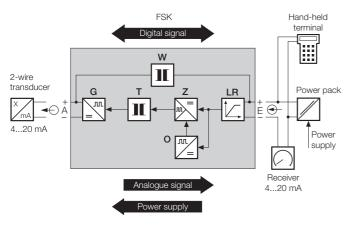
Fig. 3. Block diagram.
