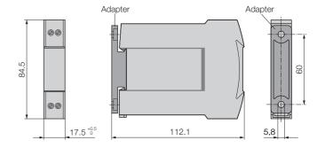
Fig. 7. SINEAX SI 815-5.... (housing **N17**) with adapter for wall mounting.
