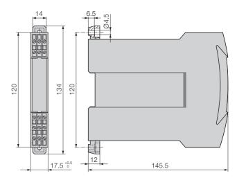
Fig. 8. SINEAX SI 815-1.... (housing **\$17**) clipped onto a top-hat rail  $(35 \times 7.5 \text{ or } 35 \times 15 \text{ mm}$ , acc. to EN 50 022).
